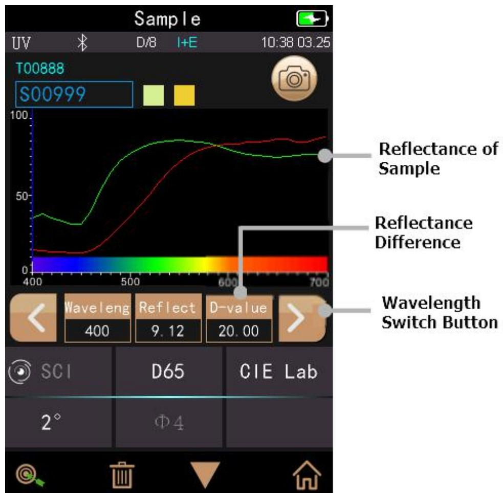
Figure 12 Reflectance of Sample Measurement
